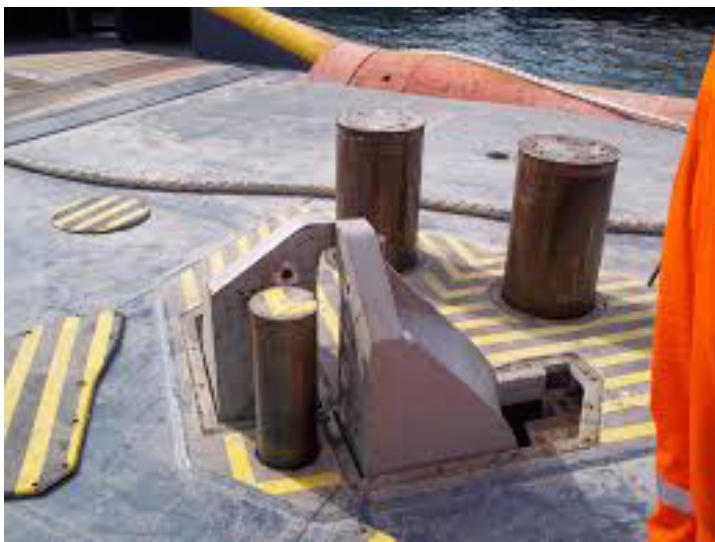
Figure 33. Shark jaws and towing pins. [Image courtesy of Wikipedia.]
