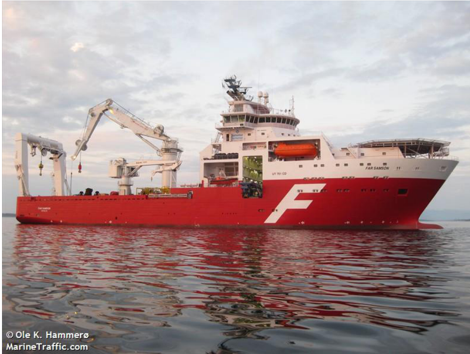
Figure 29. Far Samson, Guinness record bollard pull “tug”. [Image courtesy of Ole K. Hammero, MarineTraffic.com.]
